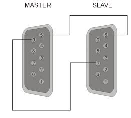
With this configuration the Master unit has ultimate control over slave unit.
